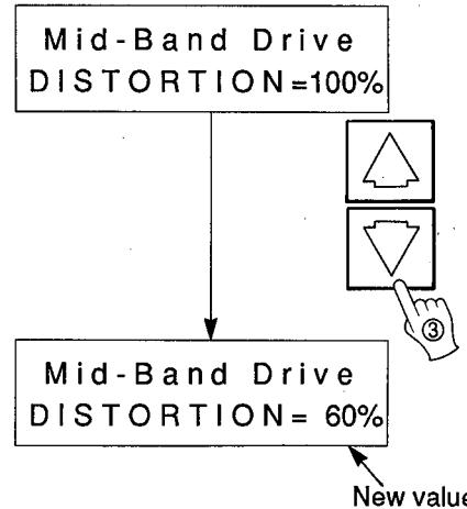
In this way you can go through and edit any number of the parameters to create the sound you want. If, however, you select and recall a new effect without first storing your edited parameters in a memory location between 51 and 00, any changes you have made will be lost and will have to be re-programmed. If you want to keep an edited effect, use the STORE operation described below.
