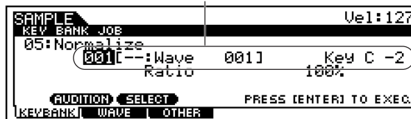
Set the Waveform and Key Bank containing the sample to be normalized.
