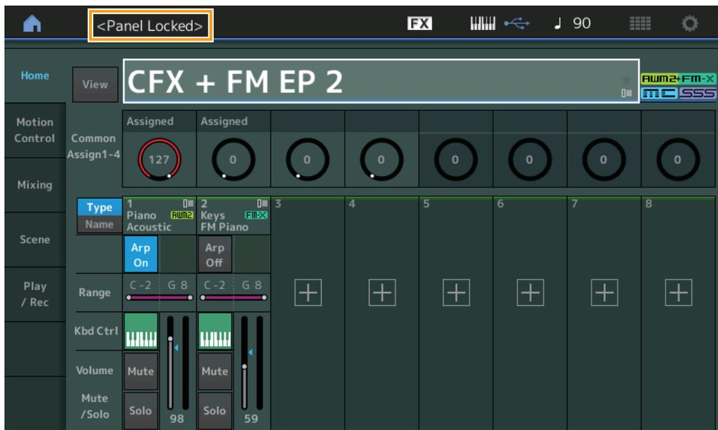
To unlock the panel, press [SHIFT] + [AUDITION] again. When the Panel Lock Function is engaged, all operations will be unavailable, except the keyboard, pedals, Master Volume, Super Knob, Pitch Bend wheel, Modulation wheel, and the unlock operation. This lock also applies to touch panel operations.
