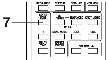
**7** Select the center channel output mode according to your speaker configuration.
