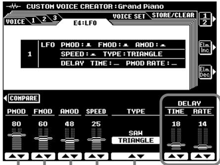
Vibrato effect based on LFO modulation, with a variable delay between the time a key is played and the beginning of the vibrato effect.
