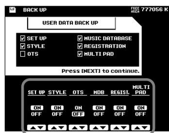
Set the data type to ON or OFF. Data types set to ON are backed up.
