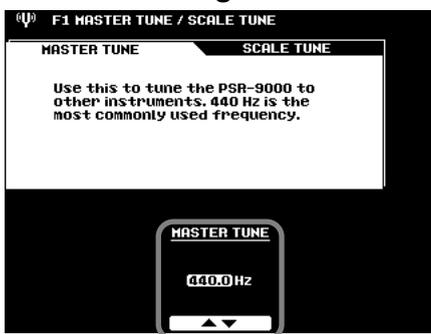
Tune the overall pitch of the 9000Pro from 414.6 - 466.8 Hz (referenced to A3). A3 = 440 Hz is standard "concert" pitch.
