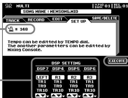
The tempo of the song can be set as required via the Data dial, and all other available parameters can be modified as required via the MIXING CONSOLE displays.
