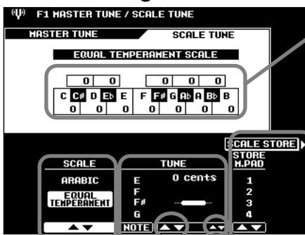
The current tuning of each note is shown in the corresponding key.
