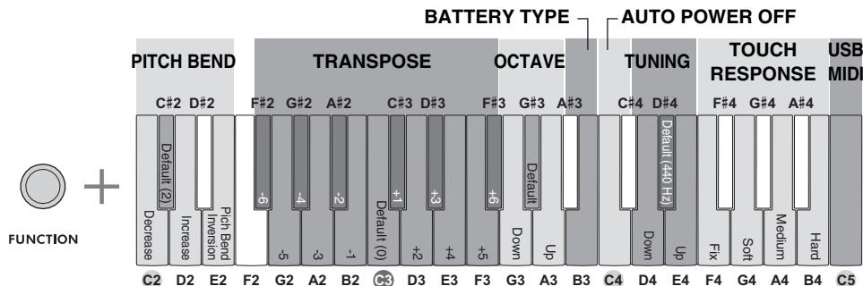
The label below each key in front of the instrument shows the function of the key when used with the [FUNCTION] button.
