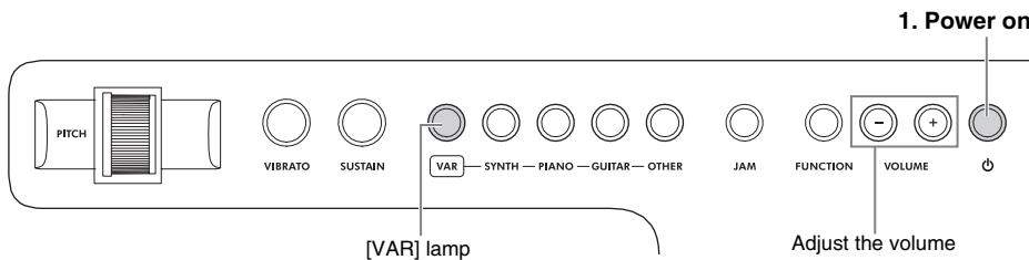
The [VAR] lamp is lit in red when the power is on.
