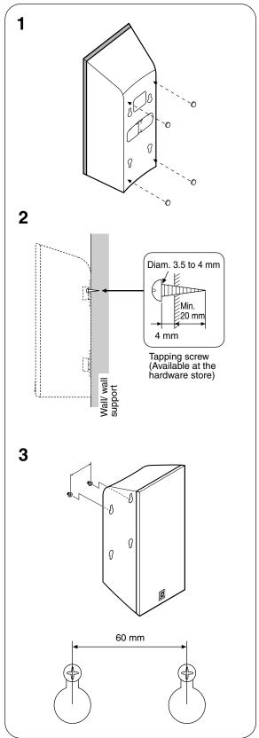
Mount the rear speakers on a shelf, rack or directly on the floor, or hang them on the wall.
