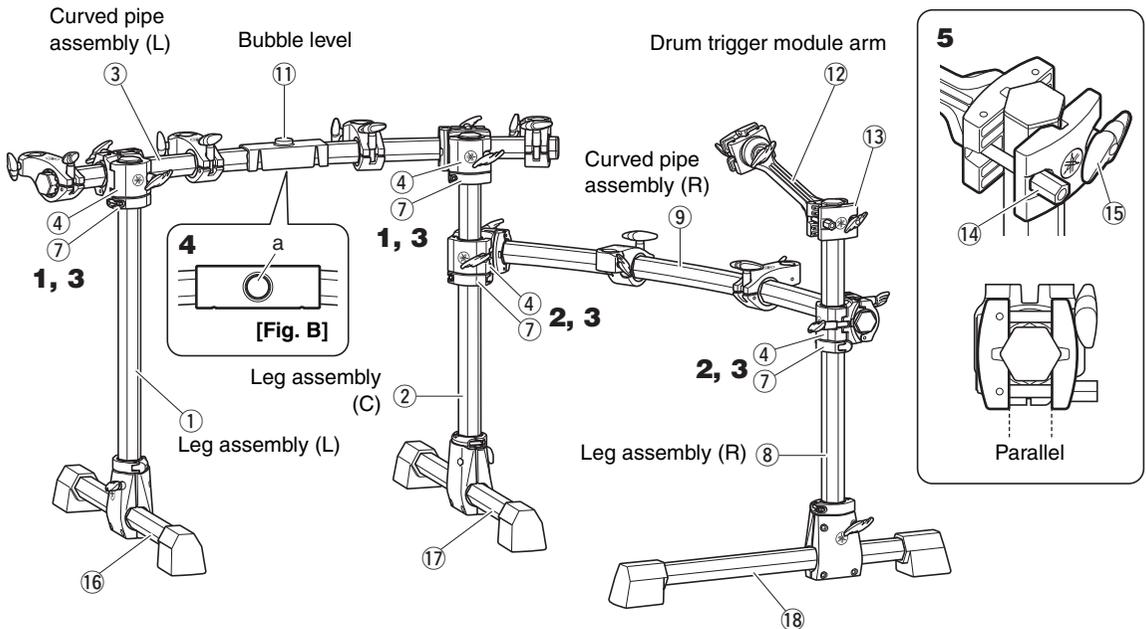
1. Attach the curved pipe assembly (L) (3) to the leg assemblies (L) (1) and (C) (2) and secure. Loosen the fixing bolts (5) on the open clamps (4) attached to both ends of the curved pipe assembly (L) (3), then align the sleeve (6) and memory clamp (7) on the leg assemblies and attach. When attaching, make sure that the nub on the memory clamp (7) is aligned with the indent on the open clamp (4) (Fig. A).
