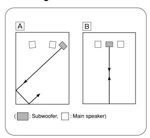
It is recommended to place the subwoofer on the outside of either the right or the left main speaker. (See fig.  $\boxed{\mathbb{A}}$ .) The placement shown in fig.  $\boxed{\mathbb{B}}$  is also possible, however, if the subwoofer system is placed directly facing the wall, the bass effect may die because the sound from it and the sound reflected by the wall may cancel out each other. To prevent this from happening, face the subwoofer system at an angle as shown in fig.  $\boxed{\mathbb{A}}$ .
