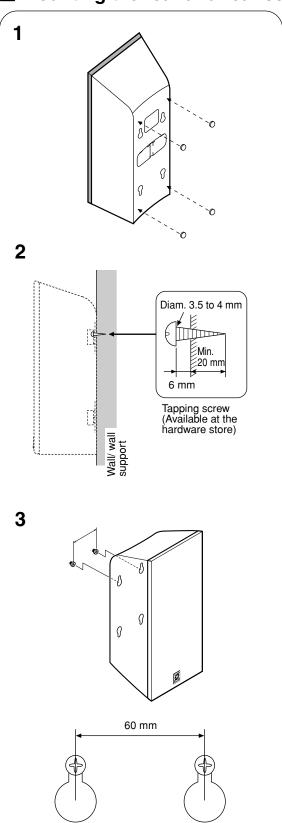
Mount the rear and rear center speakers on a shelf, rack or directly on the floor, or hang them on the wall.
