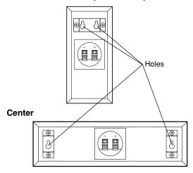
1 Fasten two screws into a firm wall or wall support at the interval shown below.
