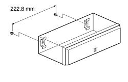
You can mount the main, rear and/or center speakers (and/or rear center speaker for NS-P436) on a wall.
