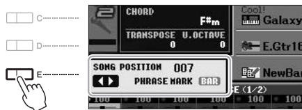
For Songs containing Phrase Marks You can switch between BAR and PHRASE MARK by pressing the [E] button.
