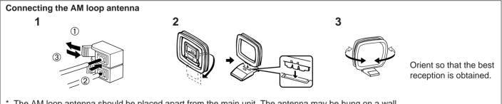
\* The AM loop antenna should be placed apart from the main unit. The antenna may be hung on a wall.
