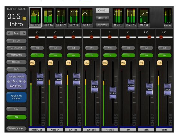
The large [MIX ON FADERS] button displays the currently selected Mix or Matrix Bus number and its name. The colour of this button matches those used in the QL console.
