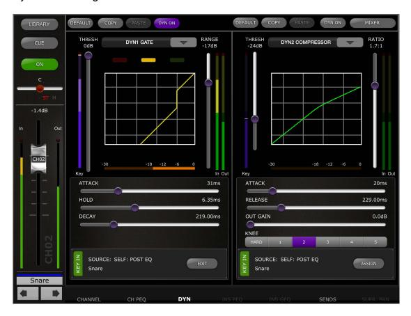
The left side of this screen (Channel Strip) is identical to the EQ Editing screen with channel fader, On button, Cue button, input and output meters, channel name, colour and navigation buttons.
