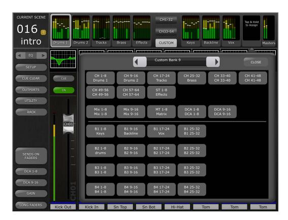
Left/Right navigation buttons can be used to navigate to other meter blocks without leaving the assignment pop-up. To exit the assignment pop-up, touch anywhere outside of the pop-up or touch the close button in the top right corner.
