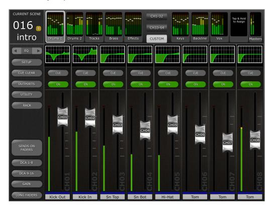
To assign a fader bank to a meter bridge block, touch and hold on a fader/meter block. An assignment pop-up menu will be displayed which contains a list of all available fader banks for the connected console model, including all standard fader banks, DCA banks and Custom Fader Banks. Touch the desired fader bank to assign it to the chosen fader block. Repeat this operation to assign multiple fader banks to the available meter bridge blocks.
