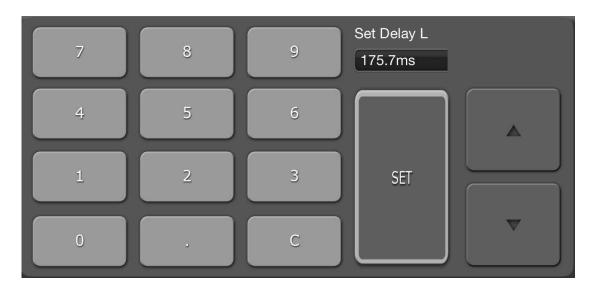
Tap the button to open the number keypad. Tap the Up/Down cursor buttons to adjust the parameter value one step at a time. The value will be sent to the console each time the cursor button is tapped.
