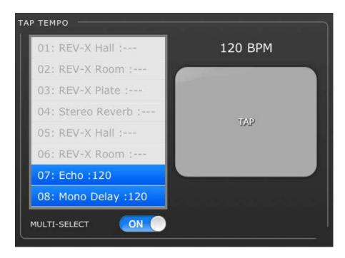
Select the relevant effect from the list of 8 effects in the left side of this section. Effects which do not have a BPM parameter will be greyed out and cannot be selected.
