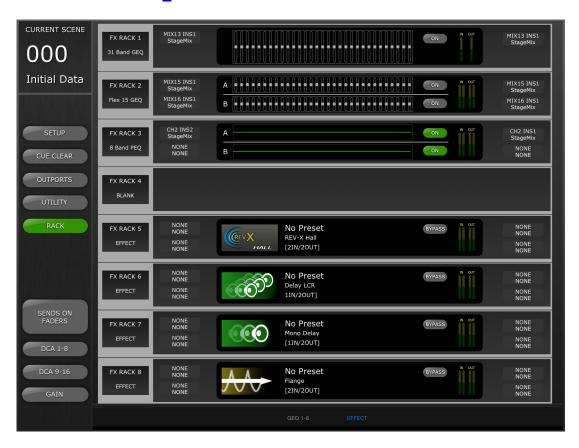
Tabs at the bottom of the screen provide access to the GEQ 1-8 and the EFFECT racks.
