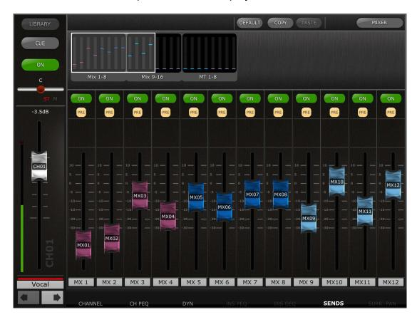
Use the meter bridge to swipe horizontally to view higher or lower numbered Mix/Matrix sends.
