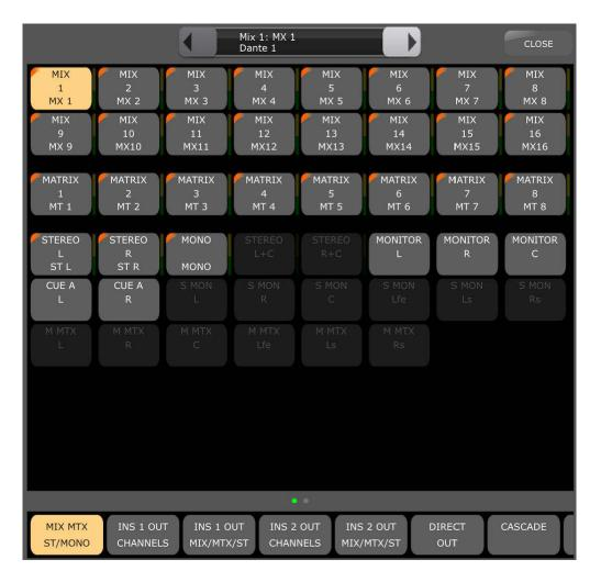
The grid displays each output channel with its type and number shown on each button. If a name has been assigned to the channel, it will also be displayed along with the channel colour where valid. For Mix/MT/Mono/ST output bus types, output metering is shown to the left of each button.
