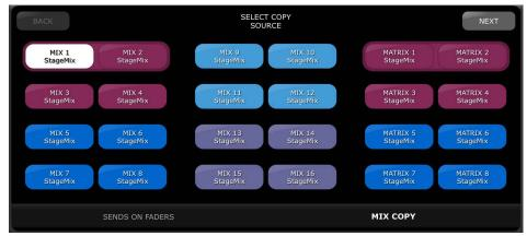
First, choose the source Mix Send to be copied, the selected Mix Send will then be highlighted in White. Touch the [NEXT] button and select the target Mix Sends to copy to. Multiple Mix Sends can be selected for targets. Touch [Next] to access the Mix Copy confirmation view. The source and target Mix Sends will be listed as selected in the previous steps. Choose whether the Copy is to include 'With Module Parameters' (Output Mix/MT channel settings) and/or 'With Mix Sends
