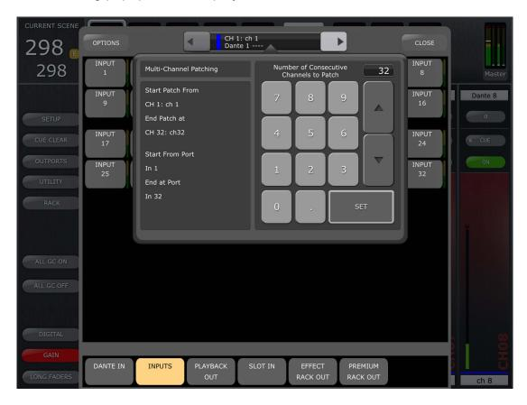
Using the keypad, enter the required number of consecutive channels to be patched. On the left-side of the popup, the start and end channel for the multichannel patch will be displayed, along with the start input port and the end input port. Touch OK to perform the patch and a confirmation message will be show, which outlines the total patch operation which will be performed. Touch YES to continue with the Multi-Channel Patch, or NO to return to the Multi-Patch popup.
